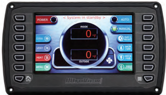
UltraView displays can be programmed to display a wide variety of vehicle functions such as climate control.
