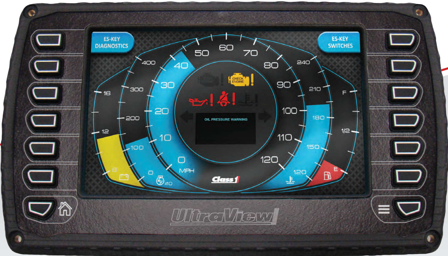
UltraView displays can be programmed to display a wide variety of vehicle functions such as climate control.
