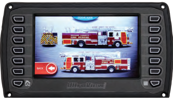
Optional touch screen display provides both screen and actual switch control for an intuitive and functional display layout.
