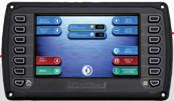
UltraView uses LCD bonded technology for the most visible display even in direct sunlight. Screen can be adjusted for night vision also.
