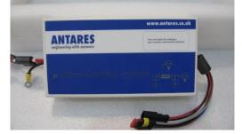
Active battery equalisation allows the "centre tap" on a battery bank to be utilised without damage to the battery bank and provide balancing of 24V battery pair when a 12V load is being powered.
