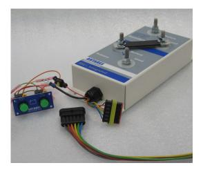
The ASC+ integrated contains all the elements of the ASC+ Dual, but is packaged for easy bulkhead mounting. It is also designed to allow multiple units to be easily combined into a more complex package. It minimises installation time, thereby saving money. The internal preprogrammed controller operates two highpower latching contactors in a variety of ways.
