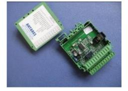
Five programmable expansion modules, provide additional control and communication ability between the individual parts of an Antares auxiliary power system, the chassis and other vehicle systems
