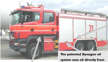
The patented Dynagen oil system uses oil directly from the ALLISON Transmission - no need for a separate oil tank.
