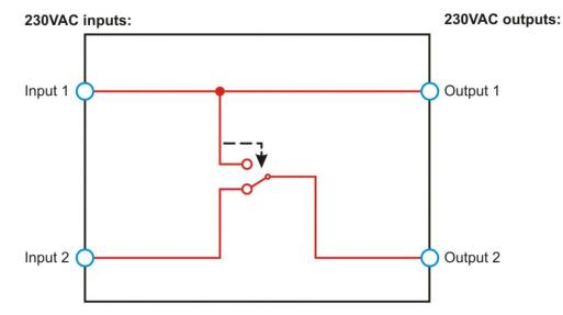
Output 2 is fed from the transfer switch, which is powered from input 2, unless input 1 is present. When input 1 is present, it is always routed through to output 2, & so is called the primary, or priority input.
